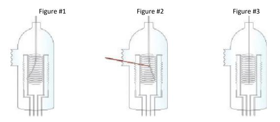
Problem: During shipment ion gauge collector wire can become displaced outside the grid. (Figure #1) Solution: You can repair the problem yourself in less than a minute by following the steps below.
