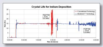
INFICON ModeLock measurement technology provides significantly longer crystal life, illustrated here in the deposition of indium.
