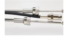
3) **QISLockAdjustableFerrule**: Using the same affixing and assembly method as above, this method brazes a ferrule on the feedthrough cooling tubes and an O-ring seal on the sensor head cooling tubes. This allows repeated disconnecting of the tubes. This option has been helium leak tested to a maximum leak rate of 4x10<sup>-9</sup> std cm3/s at room temperature. However, the leak rate may increase as temperature increases due to permeation
